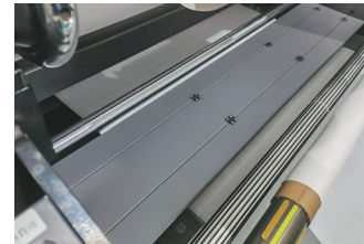
Bottom integrated heater makes the loading & take up easier, improving heating efficiency, more suitable for making samples for customer
