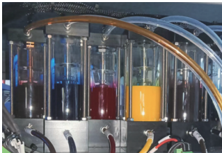
The negative pressure ink supply system is used to ensure long-term stable printing and the accuracy of the output .
